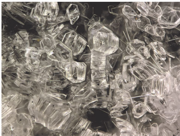
Fig. 1. Cuatrocapaite-(NH 4 ) tablets, some in vermiform stacks, with acicular torrecillasite; field of view 0.6 mm across. Specimen no. 66986.
