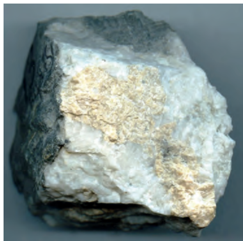
Fig. 1. Impregnation of bright colored scheelite in calcite-quartz vein. 103 × 84 mm. Central location of the Zholymbet deposit. Fig. 2. Pockets of light scheelite within gold-bearing quartz vein. 77 × 77 mm. Central location of the Bestyube deposit.
