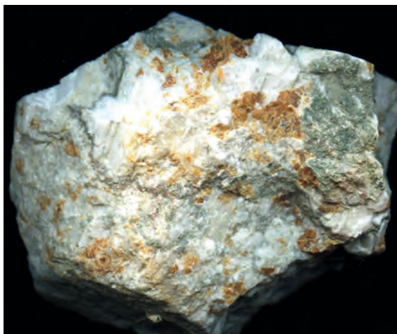
Fig. 1. Impregnation of bright colored scheelite in calcite-quartz vein. 103 × 84 mm. Central location of the Zholymbet deposit. Fig. 2. Pockets of light scheelite within gold-bearing quartz vein. 77 × 77 mm. Central location of the Bestyube deposit.
