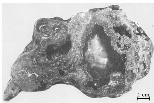
FIG. 1. Polished section of specimen № 2255-15A from an inactive chimney. Sulfides (mainly ZnS) have a zonal arrangement around the channels. The channels were cemented with epoxy resin before polishing. White irregular inclusions and fine zones are anhydrite and partly opal
