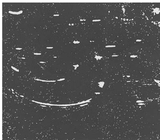
FIG. 5. Single crystal XRD ZnS pattern ( h0l ) obtained in Weissenberg camera. Curved lines with 10l and 20l indexes contain diffusion rods in reciprocal space. It is a result of the stacking faults
