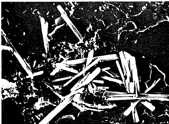
Figure 11. Barite crystals with hawleyite clumps on coaly plant fragment from Excello shale. (SEM photo; width of view is 31 \mu\text{m} .)
