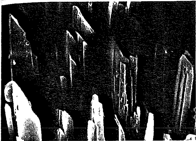
Figure 9. Corroded ferrostrunzite crystals from crust of diadochite nodule. (SEM photo; width of view is 36 \mu\text{m} .)
