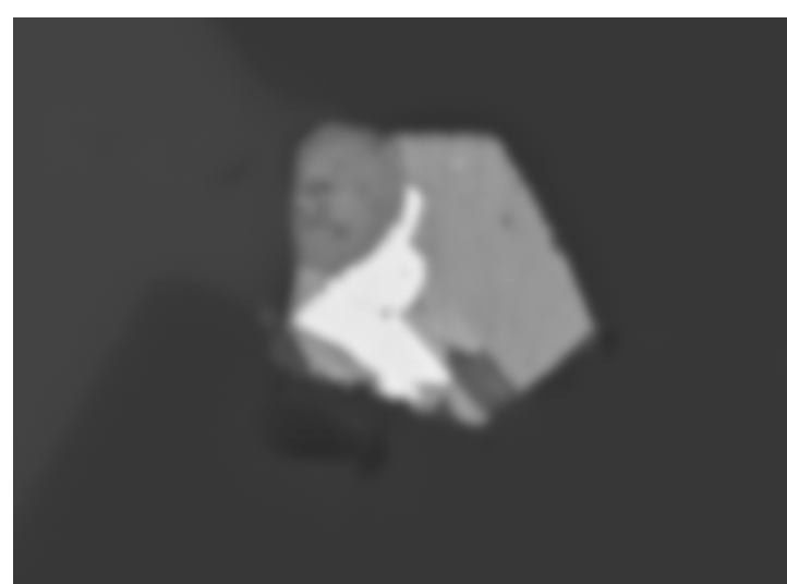
One of metal grains in grossmanite. Phases: a) Mo b) (Ni,Fe,Ir,Pt) c) (Os,Ir,Mo,Ru) d) (Ni,Nb)
