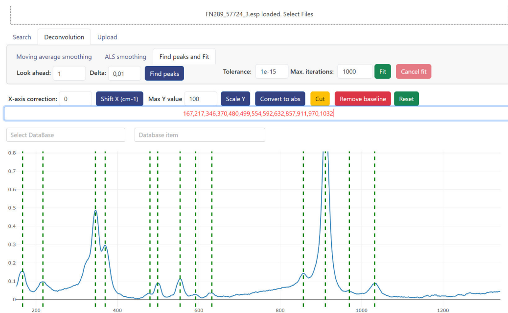
Fig. 2. Automatic peak identification on the Raman spectrum of almandine (sample FMM_1_57724).
