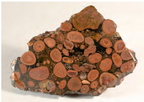
Fig. 6. Crust of residual bauxite on fresh gabbro. Quesigua, Cuba. 9 x 7 cm. FMM #VF266. Photo: M.B. Leybov.
