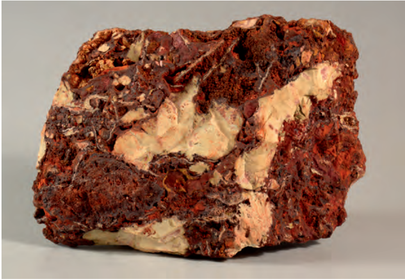
Fig. 1. Aggregates of porcelainous gibbsite in hematite and residual bauxite (developing after basalt), central India, 14.5 x 9.5 cm. FMM # 92368. Photo: M.B. Leybov.
