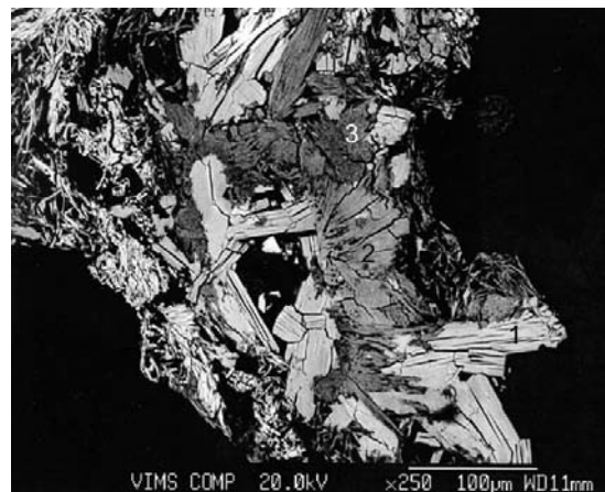
Fig. 5. Heterogeneous structure of a grain of calcurmolite, in which the crystals of uranophane with different degree of alteration prevail (the most perfect are white (1), less perfect are light grey (2), and still more altered are grey (3)); at the periphery of a grain the fibrous calcurmolite grow.
