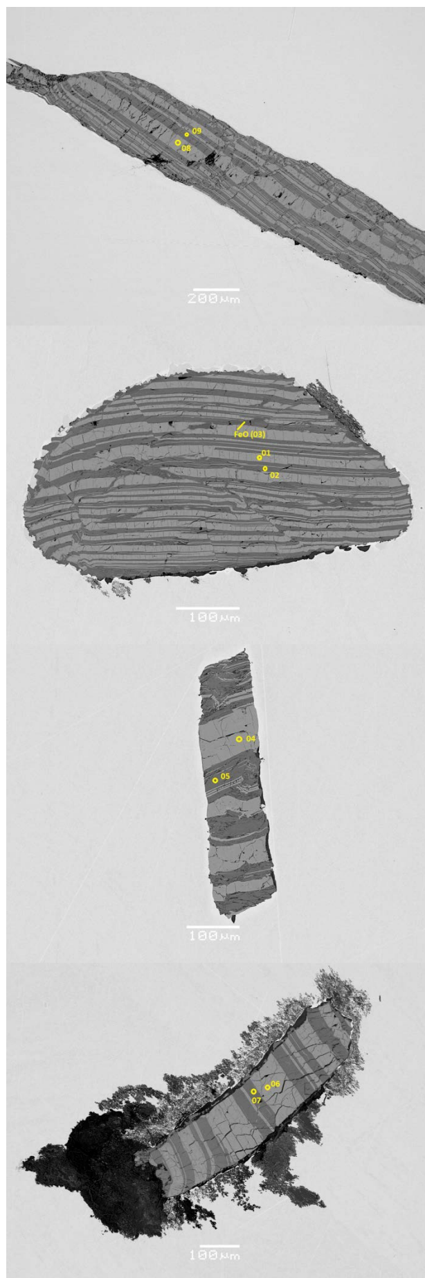
Fig.2 Daubreelite-troilite lamellar aggregates in plessite matrix.
