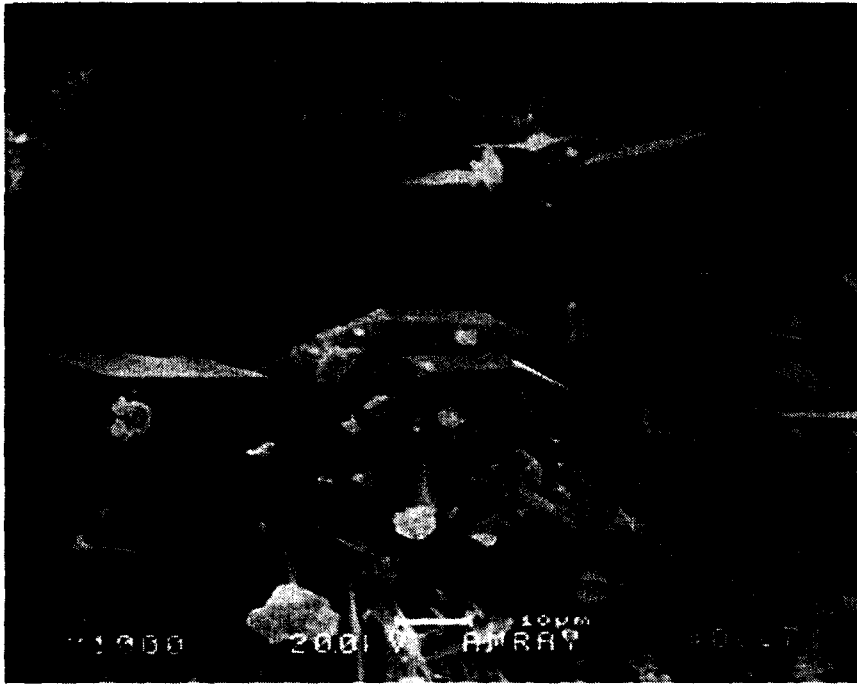
Fig. 3. Scanning electron photomicrograph of authigenic calcite (rhomboids) and abelsonite crystals (plate-like) from the ERDA/LERC SUB 12 core hole, Uinta Basin, Utah.
